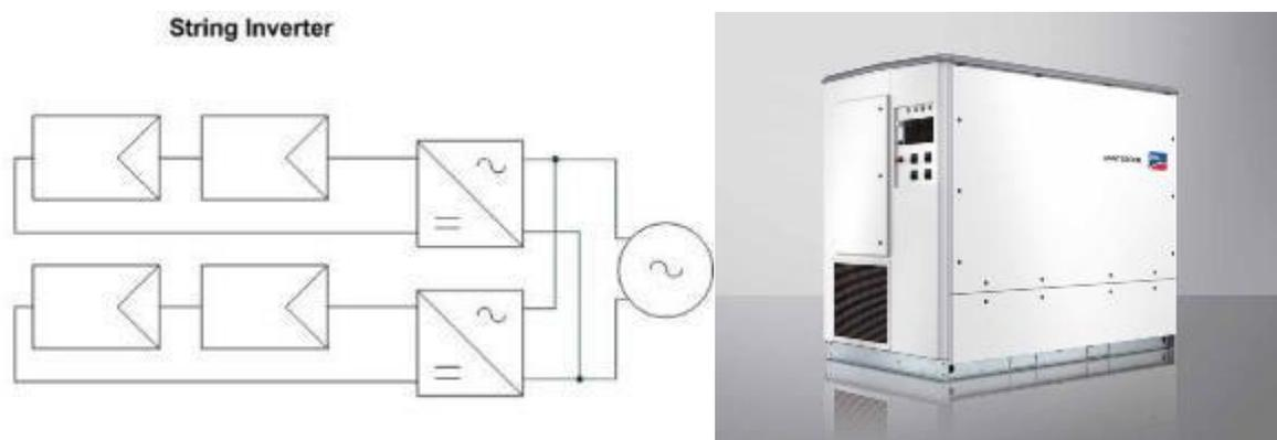
**Figure 3-16: String Inverter Connection Concept (right) and Exterior.**
