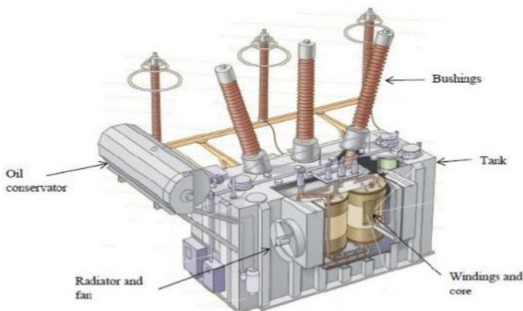
**Figure 3-17: Major Components of a Liquid-Immersed Power Transformer**
