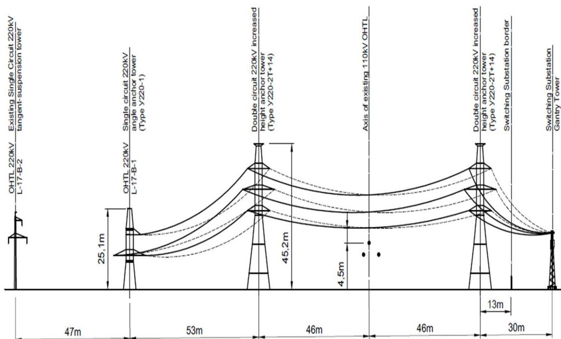
Figure 3-20: New overhead line between site and grid connection
