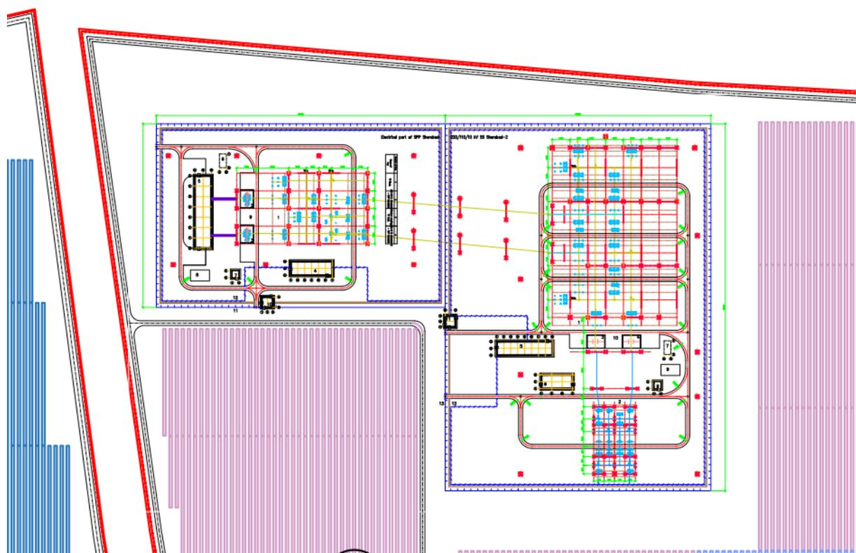
**Figure 2-10. Location of on-site substation**
