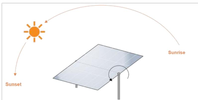
Figure 2-5. Schematic Diagram of Single-Axis Tracking System
