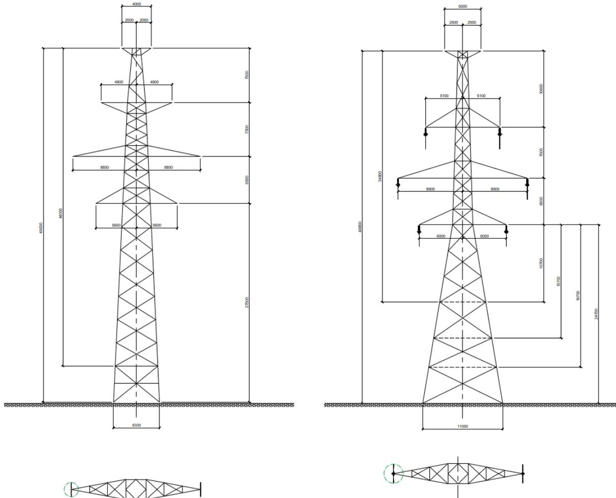
**Figure 2-20. Steel lattice towers for the overhead line**
