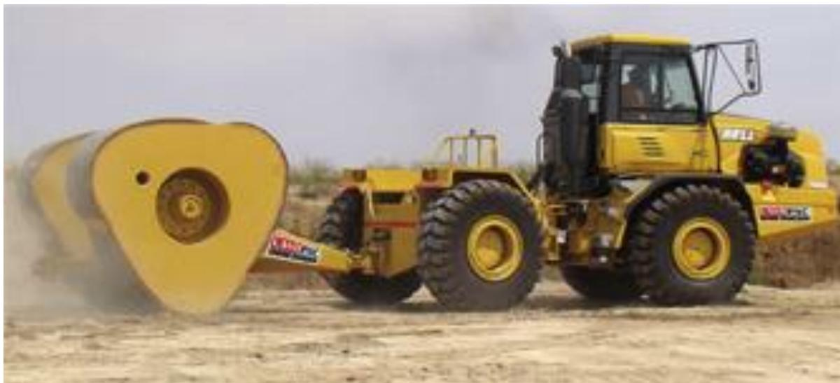
**Figure 2-22. Rolling dynamic compaction (RDC)**
