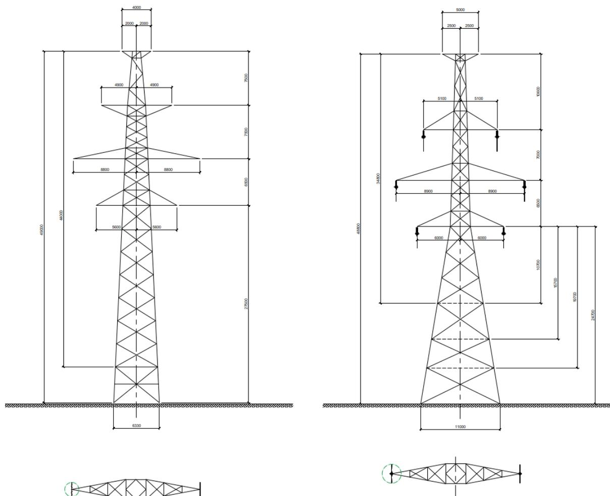
**Figure 2-12. Steel lattice towers for the overhead line**
