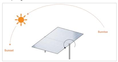
Figure 2-5. Schematic Diagram of Single-Axis Tracking System
