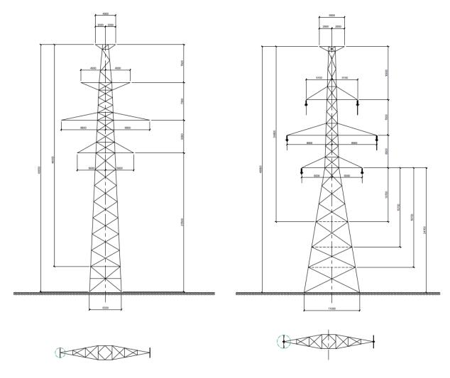
Figure 2-20. Steel lattice towers for the overhead line
