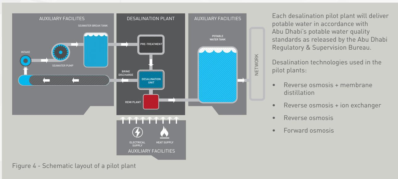
Figure 4 - Schematic layout of a pilot plant
