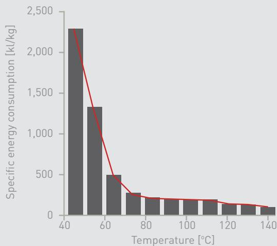
Figure 1 - Target specific thermal energy consumption of thermal desalination plants using advanced desalination technologies in dependence of the temperature of the energy supply
