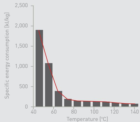
Figure 2 - Target specific thermal energy consumption of thermal desalination plants using innovative desalination technologies in dependence of the temperature of the energy supply
