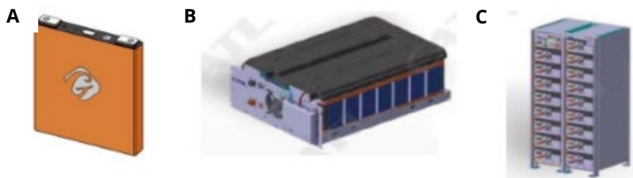
Figure 25: A: Battery cell (175×27×200mm), B: Battery Pack (contains 40 battery cells), C: Battery Cluster (contains 18 battery packs).
